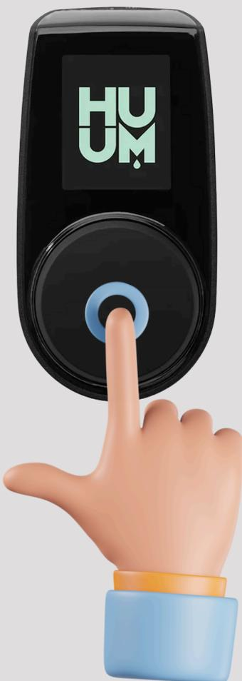
1. Press and hold the button on the HUUM control unit for 10 seconds.
