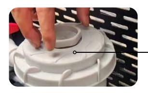
After replacing the filter element. Screw on the filter cover, open the ball valves. Then open the exhaust valve slightly to ensure there are no air locks. After this you can turn the lce bath back on
